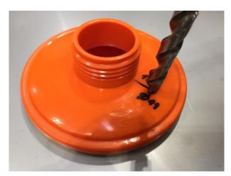
Using a suitable drill, a hole with a **10.5 mm** diameter (or with a 10mm drill, if a 10.5 mm is not available) is drilled into the cover of the fermenter directly below the sensor cable connection located on the attached airlock. We recommend a pre-drilling with a significantly smaller drill – particularly if the cover is made of stainless steel.
