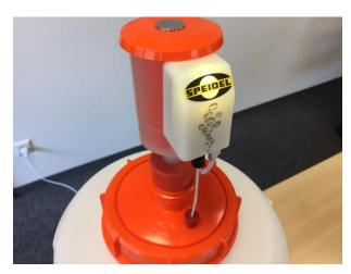
It is important that all passages into the fermenter are hermetically sealed and that fermentation gases can ONLY be discharged via the airlock. Connect the USB power cable to a power source and lay the cable so that moisture cannot run down the cable into the power supply. The LED should briefly light up in magenta and then switch to yellow (configuration mode).
